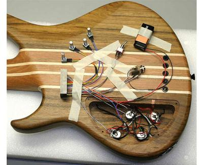
Note: it will pick up extra noise while it is out of the shielded cavity. Also note that touching the temporarily ungrounded pots or switches can cause hum.
