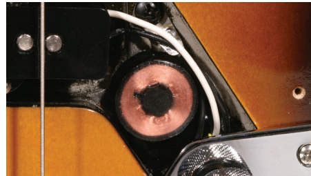
Noise Sensor installed
